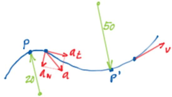
Page 51, 12-94: A car travels along a horizontal curved road that has a radius of 600m. If the speed is uniformly increased at a rate of 2000km/h<sup>2</sup>, determine the magnitude of the acceleration at the instant the speed of the car is 60km/h.
