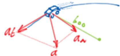
Page 51, problem 12-95: A boat is traveling along a circular path having a radius of 20m. Determine the magnitude of the boat's acceleration if at a given instant the boat's speed is  $v=5$  m/s and the rate of increase in the speed is  $dv/dt = 2$  m/s<sup>2</sup>.
